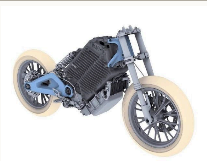
S2, STRIPPED LIVEWIRE PLATFORM RENDER
